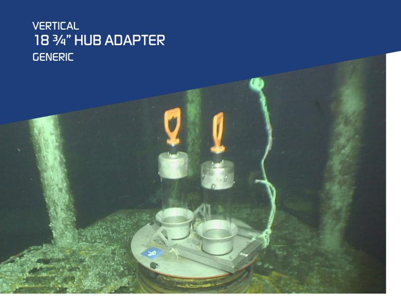
This adapter is designed for cleaning 18 %" hubs using SolidCitric. Various interface inserts can be mounted to the adapter in order to fit any 18 %" configuration. The tool is fitted with two SolidCitric cartridge slots if a large volume is required to be saturated.
